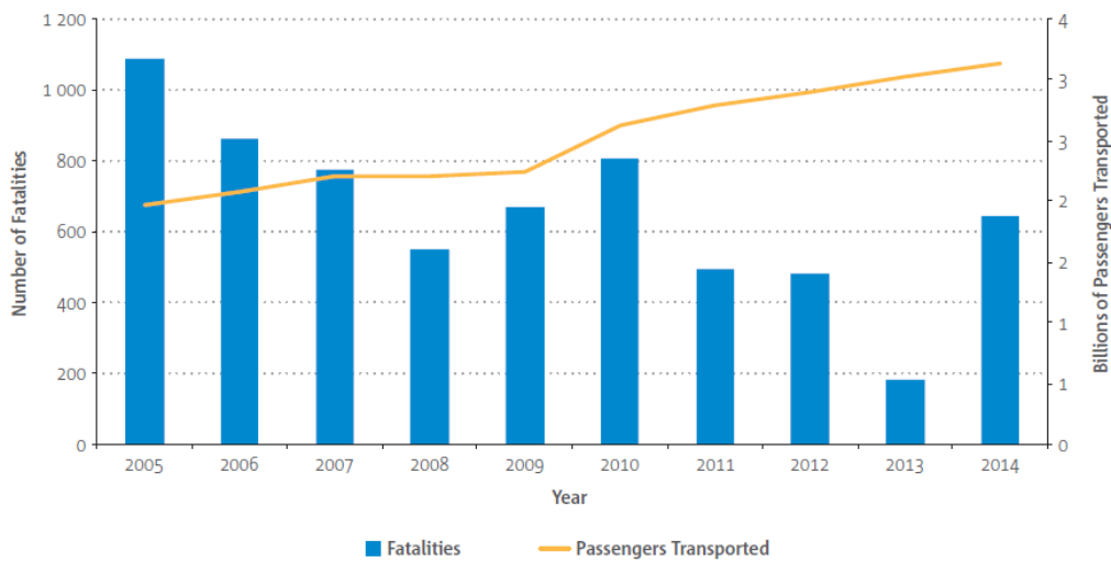
Figure 3 Number of worldwide fatalities involving passenger and cargo operations with the number of passengers transported, maximum take-off mass above 5700 kg (EASA, 2015)
