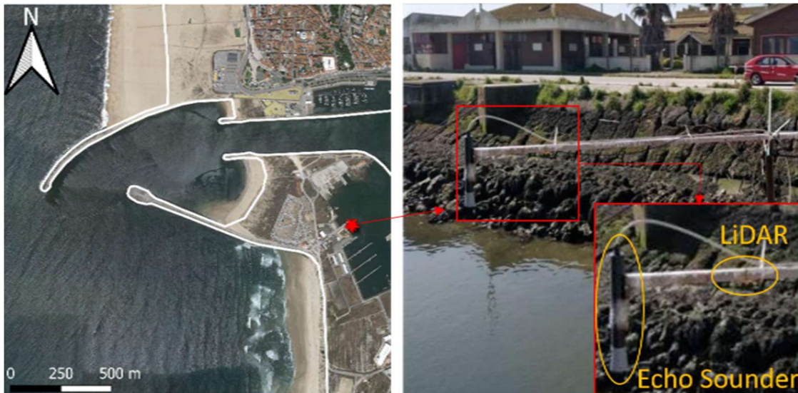
Figure 3.3 – Left: Location of the remote sensing tidal gauges within the harbour; right: perched sensors
