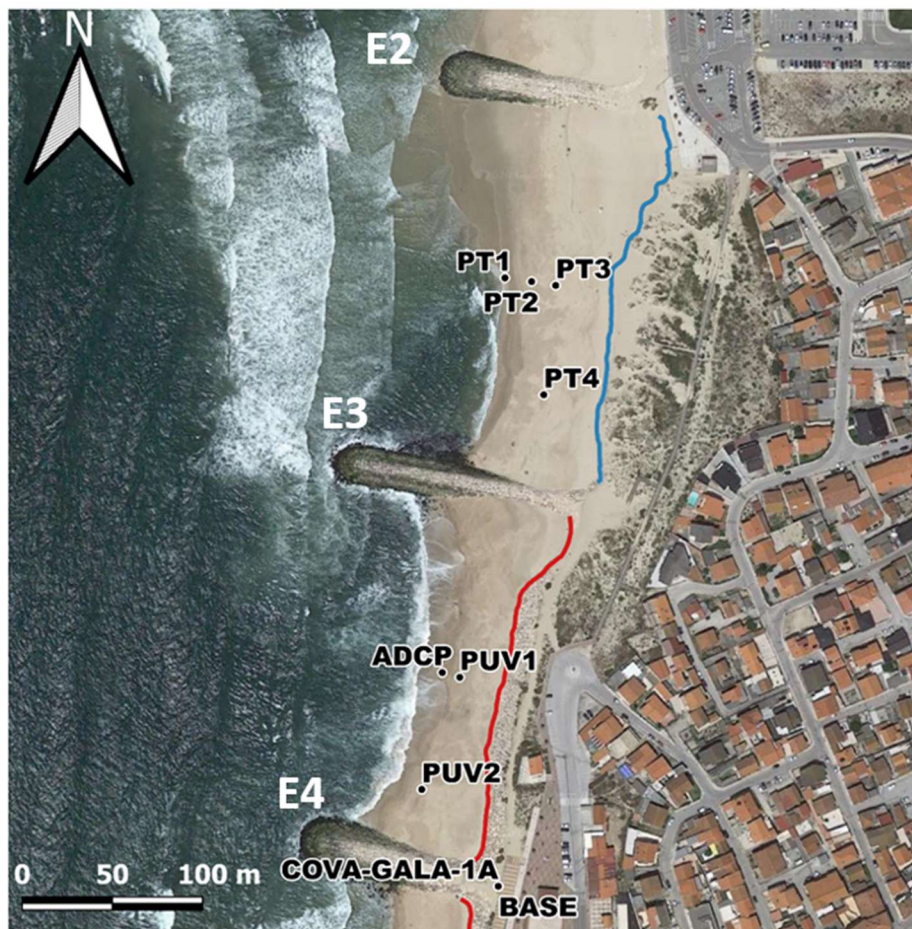
Figure 3.1 – Hydrodynamic instruments deployment at Cova-Gala: Google Satellite view of the instrumented beach cells with the position of all deployed instruments, solid lines are the respective coastlines (in blue: sand dune foot; in red: seawall toe)
