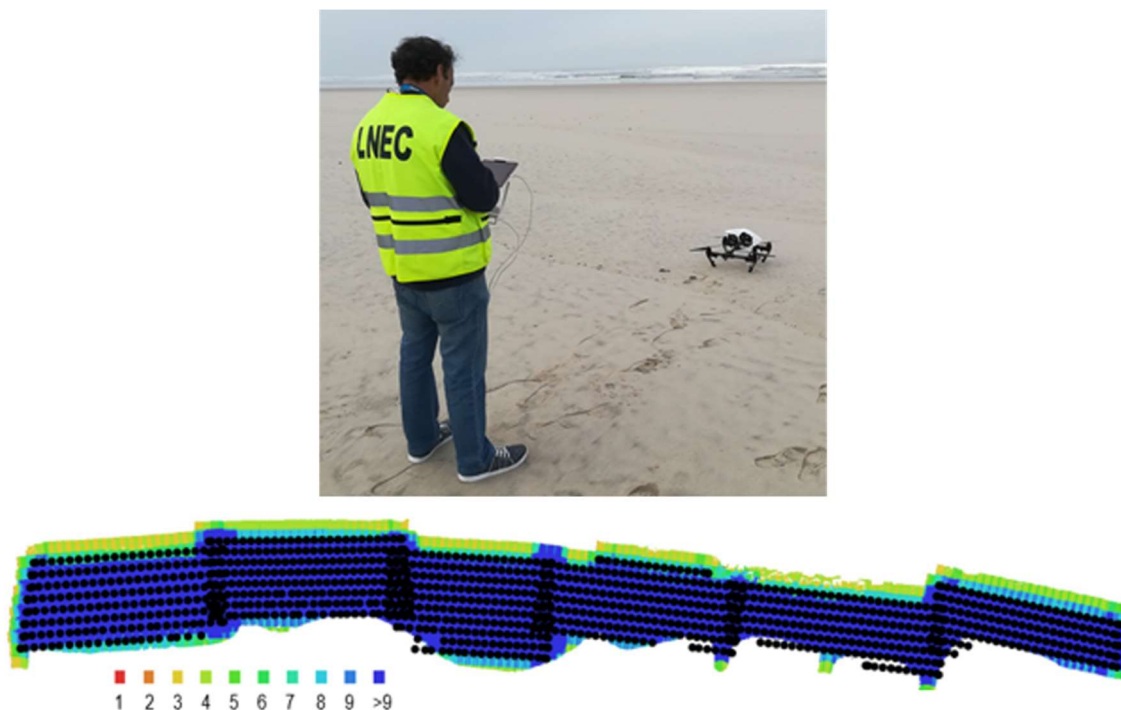
Figure 3.5 – Upper panel: drone operator; lower panel: camera locations and photo overlap during the drone survey of Cova-Gala beach on 11/Mar/2020
