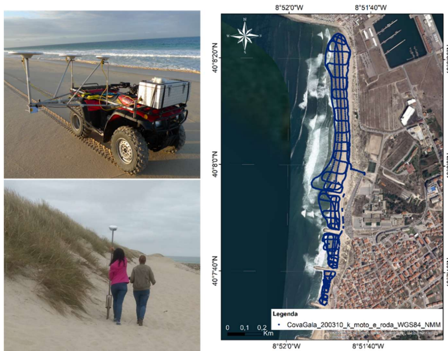
Figure 3.4 – Quad survey. Upper left panel: Quad-mounted GNSS antenna; lower left panel: Wheel mounted GNSS antenna; right panel: Post processed survey points
