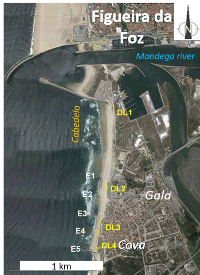
Figure 2.1 – Study area. Google Satellite view of the Figueira da Foz harbour and the coastal stretch of Cova-Gala, with its four alongshore defence structures (DL1 to DL4) and five groynes (E1 to E5)
