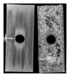
**Figure 2.** Wood borer attack on SCA-treated (**left**) and untreated control Scots pine sapwood (**right**) after four months exposure in the Oslofjord.
