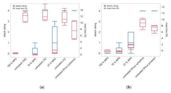
**Figure 1.** Mass loss (in red) and attack rating (in blue) of SCA-treated and untreated control wood after termite attack in (**a**) a two-choice test and (**b**) a no-choice test.
