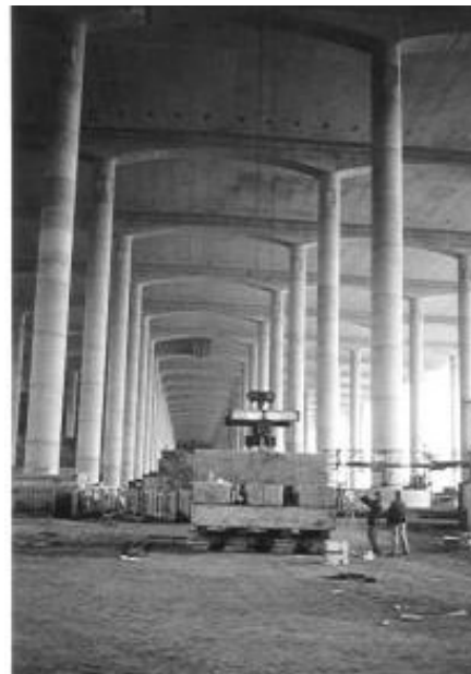
Figure17. Dynamic test - suspended weight
