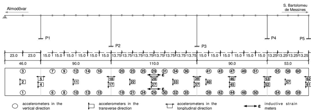
Figure 6. Scheme of the points instrumented with accelerometers in the dynamic tests.
