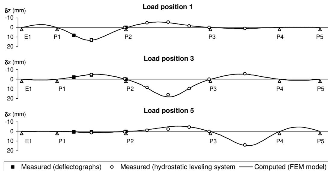
Figure 5. Comparison between measured and computed vertical displacements.
