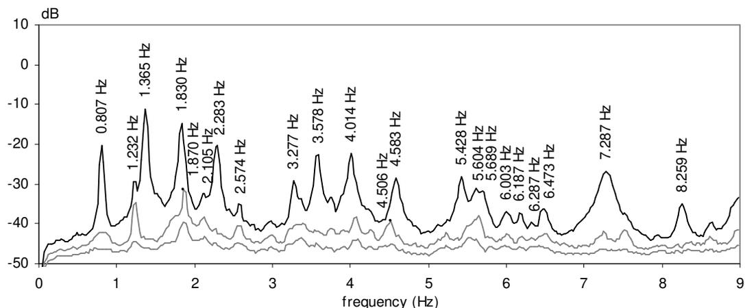
Figure 7. Spectra of singular values of the spectral densities matrix and identified frequencies.
