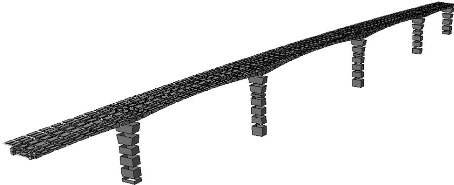
Figure 3. General view of the finite element model developed for Arade bridge.
