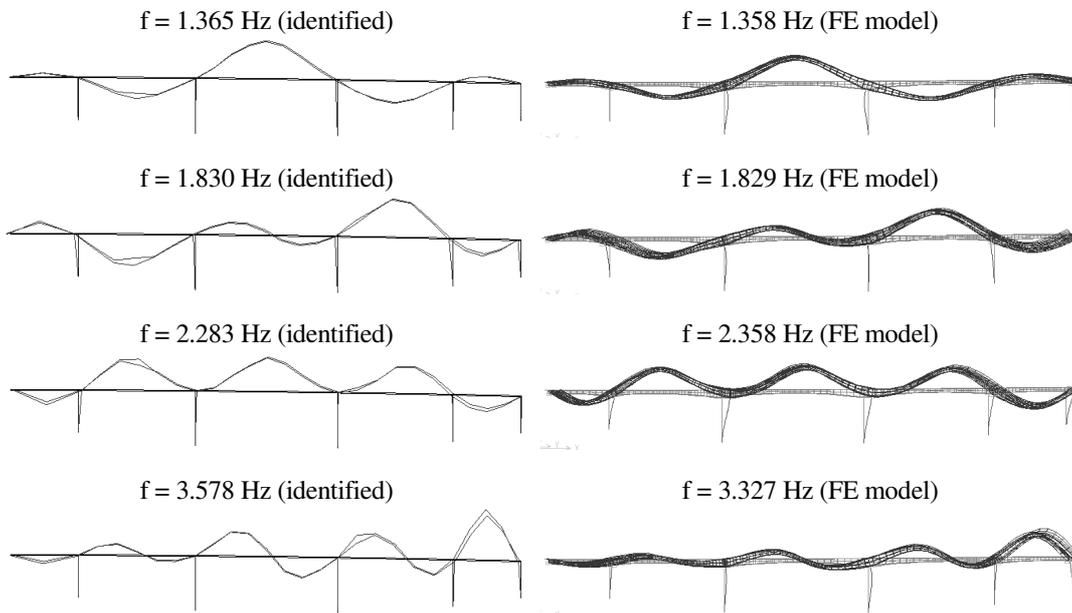
Figure 8. Identified and computed mode shapes for the first 4 vertical modes.
