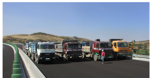
Fig. 3 Loaded lorries in use as a load test
