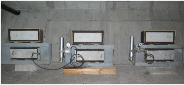
Figure 3. Creep and shrinkage specimens inside the box girder
