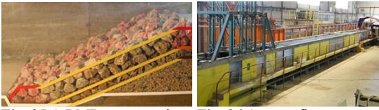
Fig. 25 A RMB cross-section Fig. 26 A wave flume
