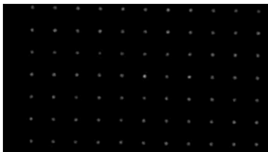
Figure 2. Observed diffraction pattern for the telephoto lens (without converter assembly).
