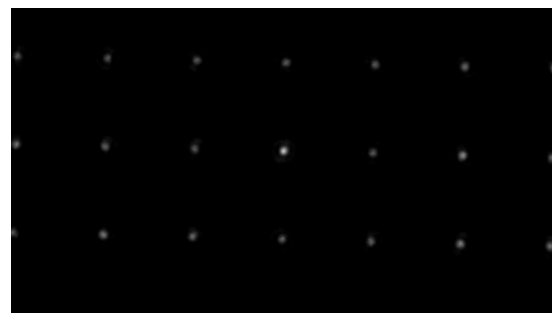
Figure 3. Observed diffraction pattern for the telephoto lens and converter assembly.
