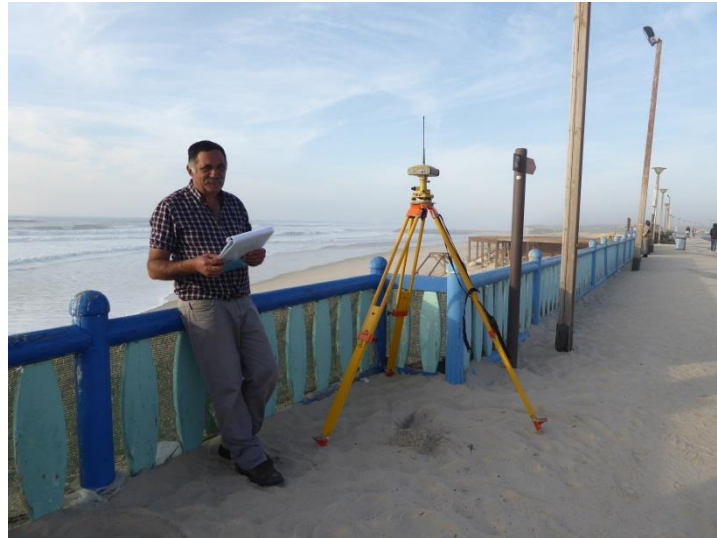
Figure 6.2 – Photograph (view towards north) of the positioning of the fixed station of the GNSS receiver on the campaign of 25/Feb/2019: pedestrian platform in front of the roundabout with the boat sculpture, north of the Sun7 Bar
