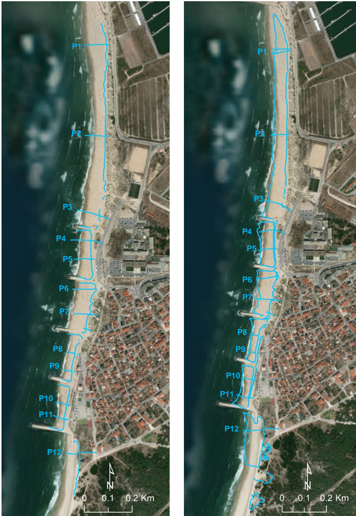
Figure 5.1 – Location of the topographic elements surveyed in Cova-Gala beach in the campaigns of 4/Feb/2019 and 21/Feb/2019, left and right, respectively. Image: ESRI Basemap
