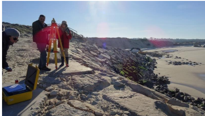
Figure 5.3 – Photograph of the positioning of the fixed station of the GNSS receiver on the campaign of 04Feb/2019: land extreme of E5; view towards south
