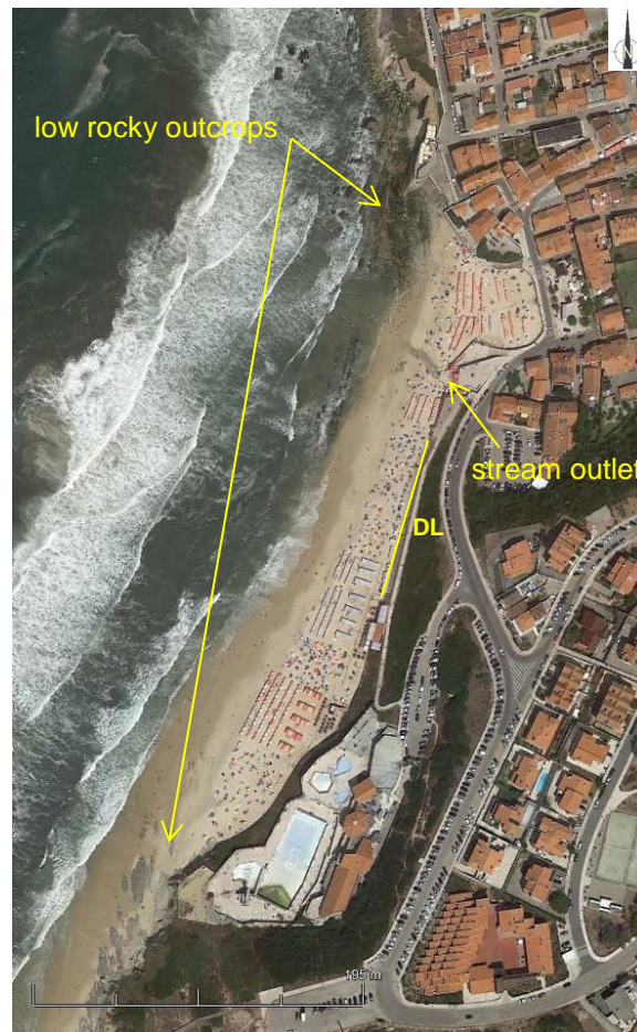
Figure 2.14 – Aerial photograph (dated of 18/8/2018; © Google Earth) of São Pedro de Moel beach and location of the low rocky outcrops, the stream outlet and the alongshore defence structure (DL)
