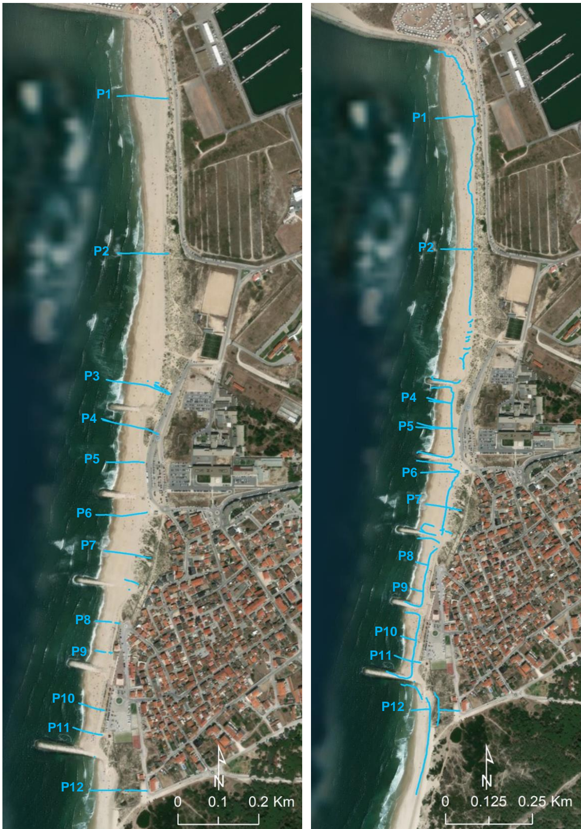
Figure 5.2 – Location of the topographic elements surveyed in Gala-Cova beach in the campaigns of 25/Feb/2019 and 26/March/2019, left and right, respectively. Image: ESRI Basemap
