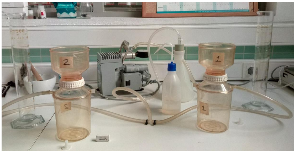
Figure 2.10 – Aspects of laboratorial procedures: filtration system used to determine suspended solids and further nutrient concentrations
