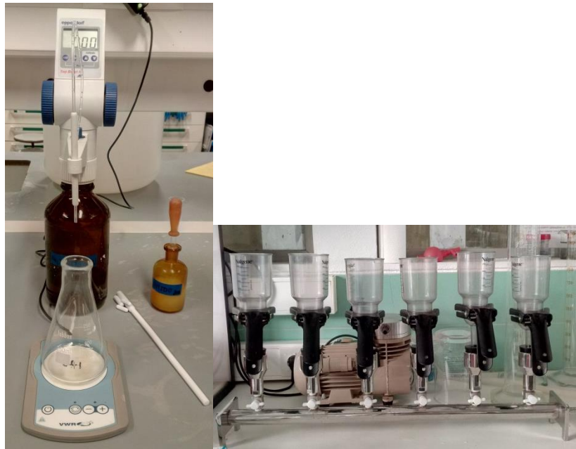
Figure 2.9 – Aspects of the laboratorial procedures: laboratorial analyses for the determination of oxygen concentration (left); filtration system used to determine the concentration of chlorophyll a (right)
