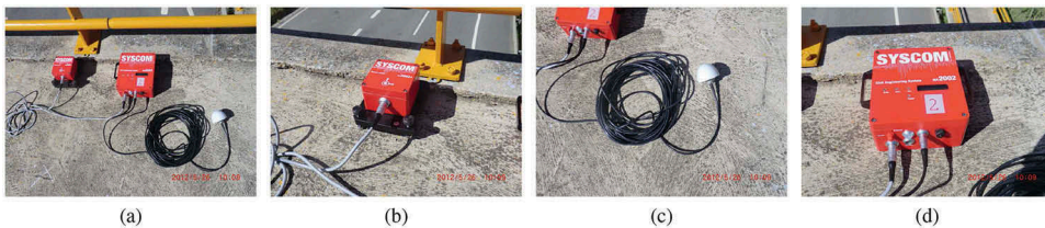
Figure 4. (a) SYSCOM MR2002-CE vibration monitoring system; (b) MS2003+ triaxial velocity sensor; (c) GPS antenna; (d) recorder.
