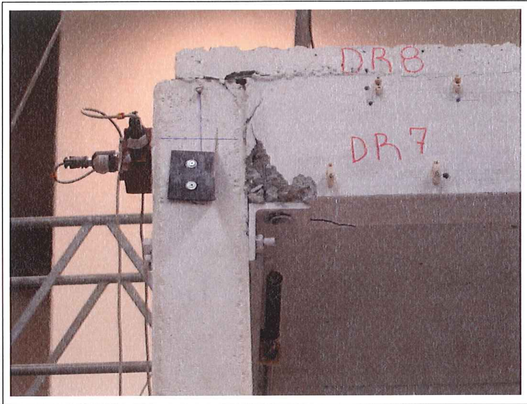
Figure F-21: Detail of the beam-column connection after the test (J9-Trans.)
