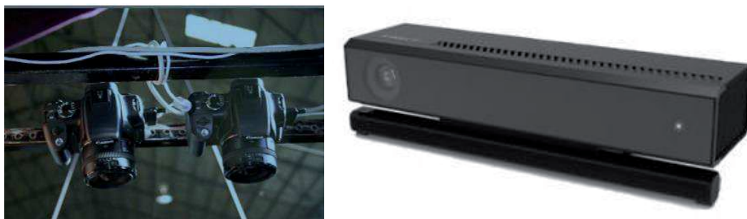
Fig. 2 Survey equipment. SLR cameras (left) and Kinect 2.0 (right)
