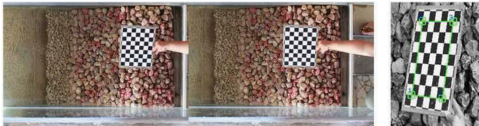
Figure 5. Example of a stereo pair and calibration board, used to calibrate the camera setup.
