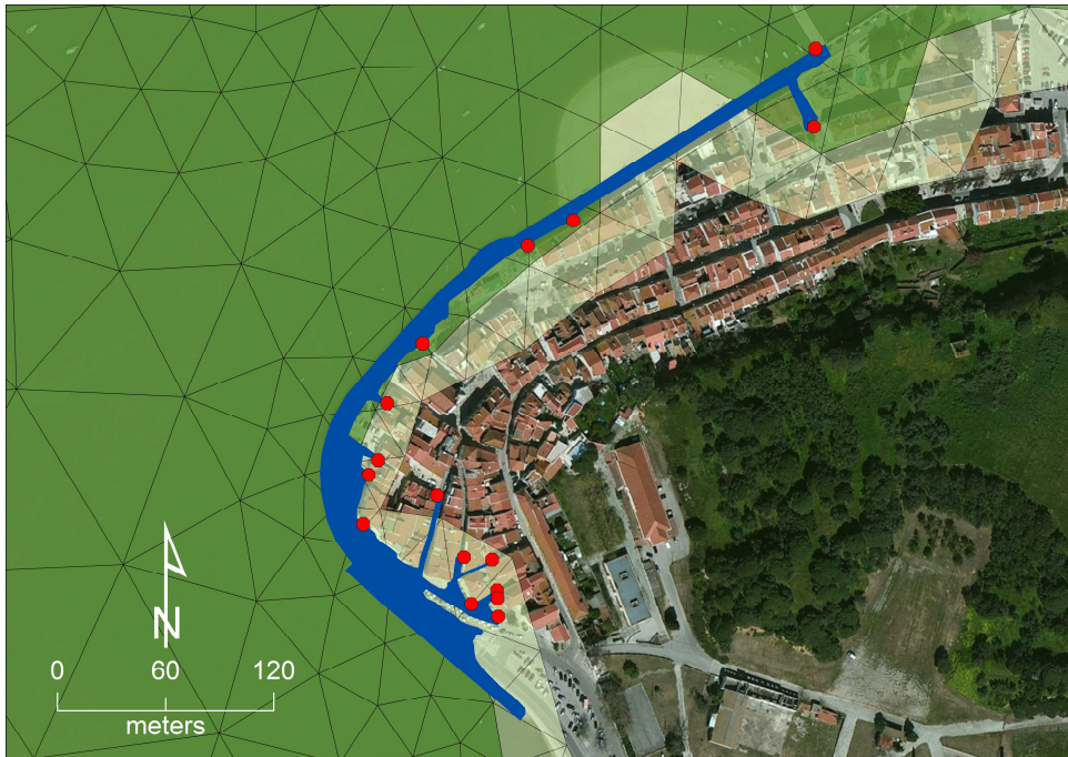
Figure 9. Validation of the modeled inundation of the Seixal downtown area during Xynthia. The red circles represent the inundation limits determined in the field and the blue shape is an interpretation of the inundated area based on those limits and the existing buildings (from Freire et al., 2016). Dark (light) green triangles represent fully (partially) wet elements as determined by the model. Fully dry elements are omitted for clarity.
