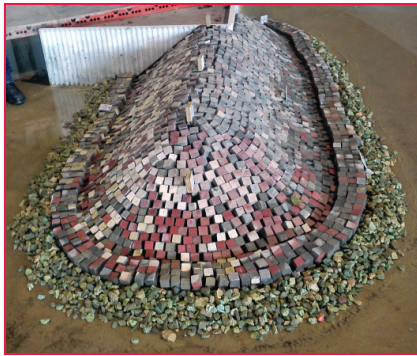
Figure 16: Model of a breakwater
