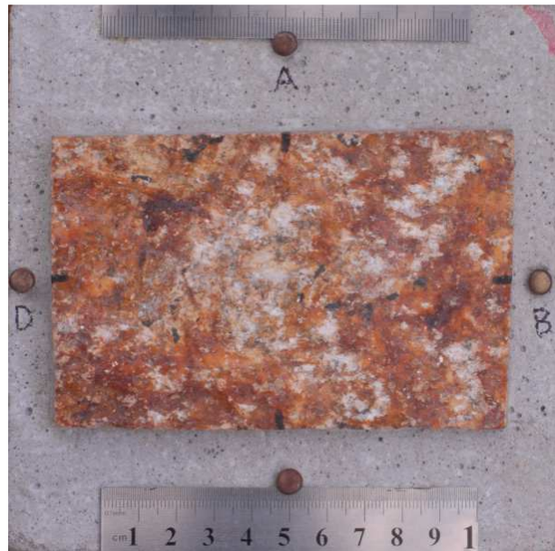
Figure 2 – Vertical photograph of one sample (12cmx8cm) of a rock embedded in a concrete block. The sample is used to characterize the mechanical properties of rocks and rocky massifs
