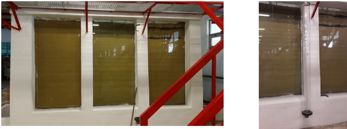
Figure 7 – Detail of three soil layers being tested simultaneously (left) and the external piezometer (right)
