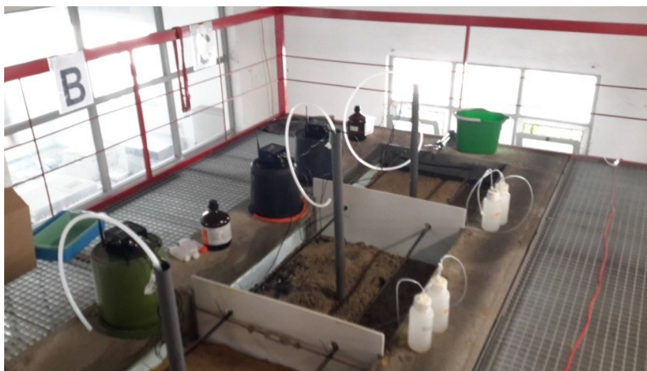
Figure 10 – In situ monitoring devices, both for the saturated and vadose zones
