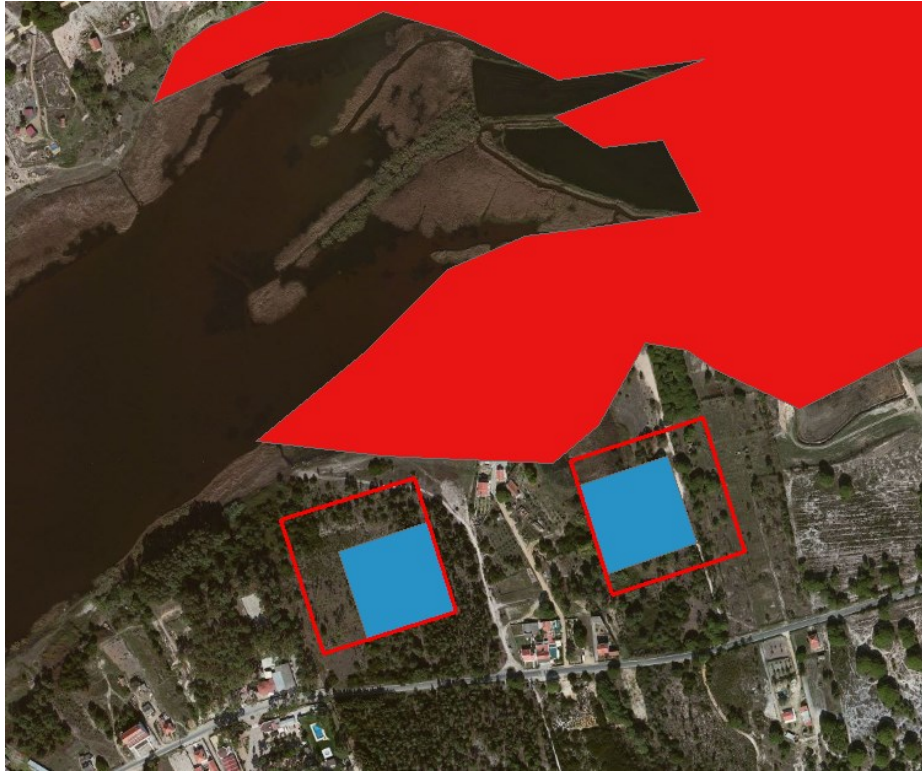
Figure 36 – Possible location for the SAT-MAR basins at Melides (blue square is 100 m side and red square is 150 m side)
