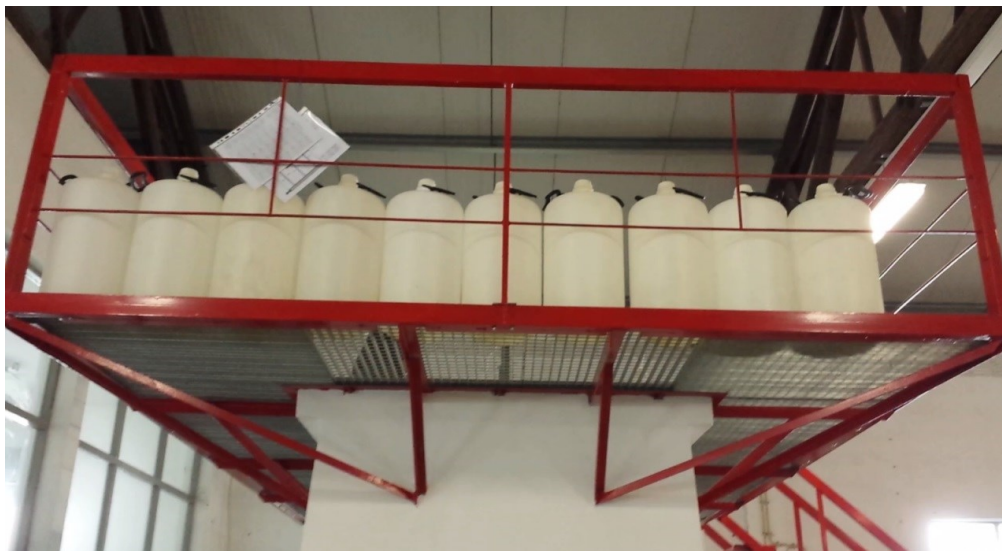
Figure 11 – Bottles used to store the tracer for the physical (sandbox) model Experiment 1
