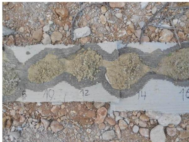
**Figure 15 – Regular sample collection of materials ("cuttings")**
