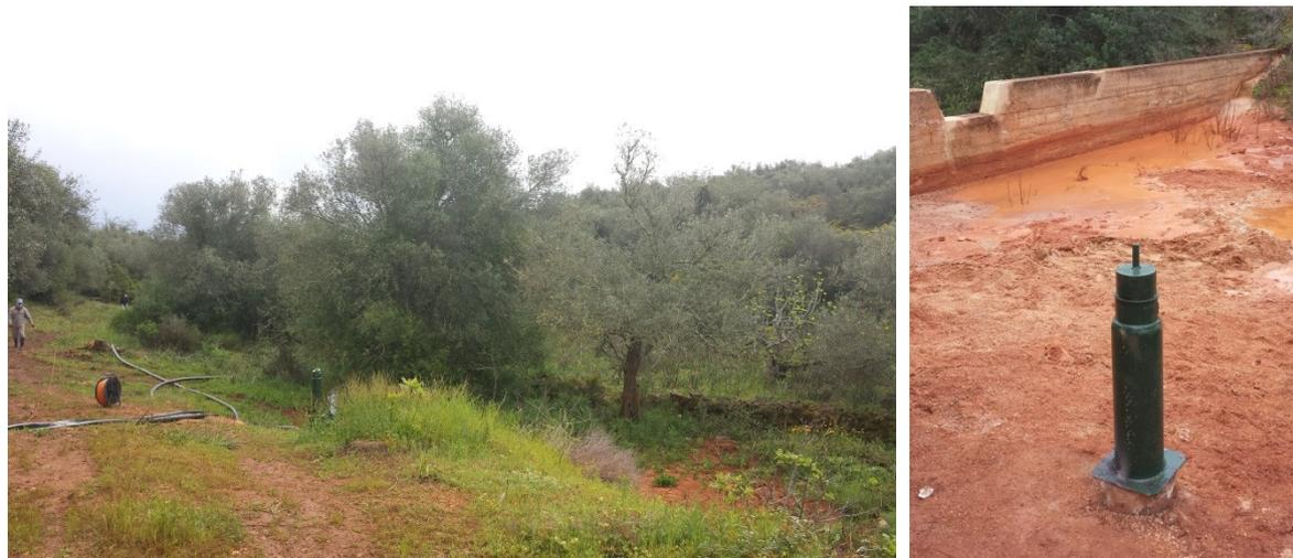
**Figure 77 – New piezometers at Cerro do Bardo. CB1 in the left and CB2 in the right**
