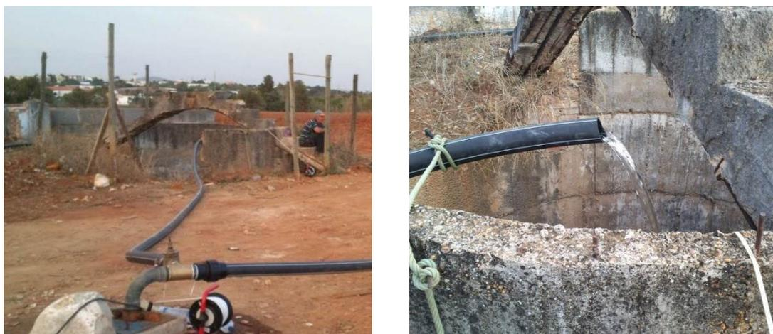
**Figure 57 – Infiltration test at DEMO site PT1\_3, injection test at a large diameter well. The pumping well can be seen on the bottom of the left picture**
