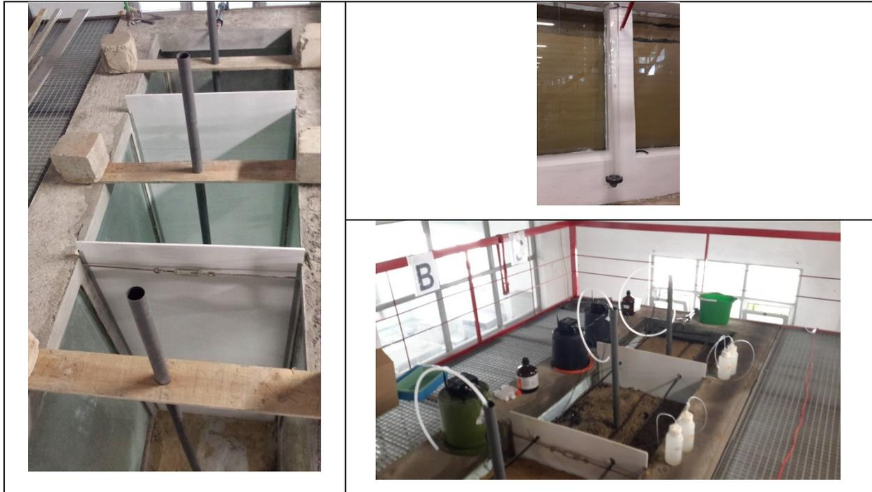
Figure 98 – LNEC physical (sandbox) model sections, A, B and C
