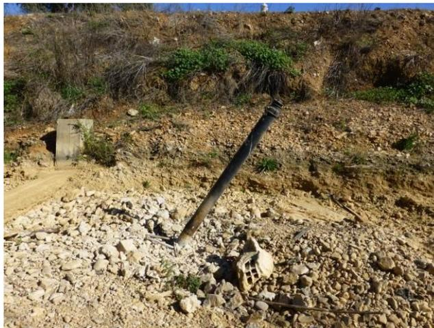
Figure 6 – LNEC1 piezometer before rehabilitation
