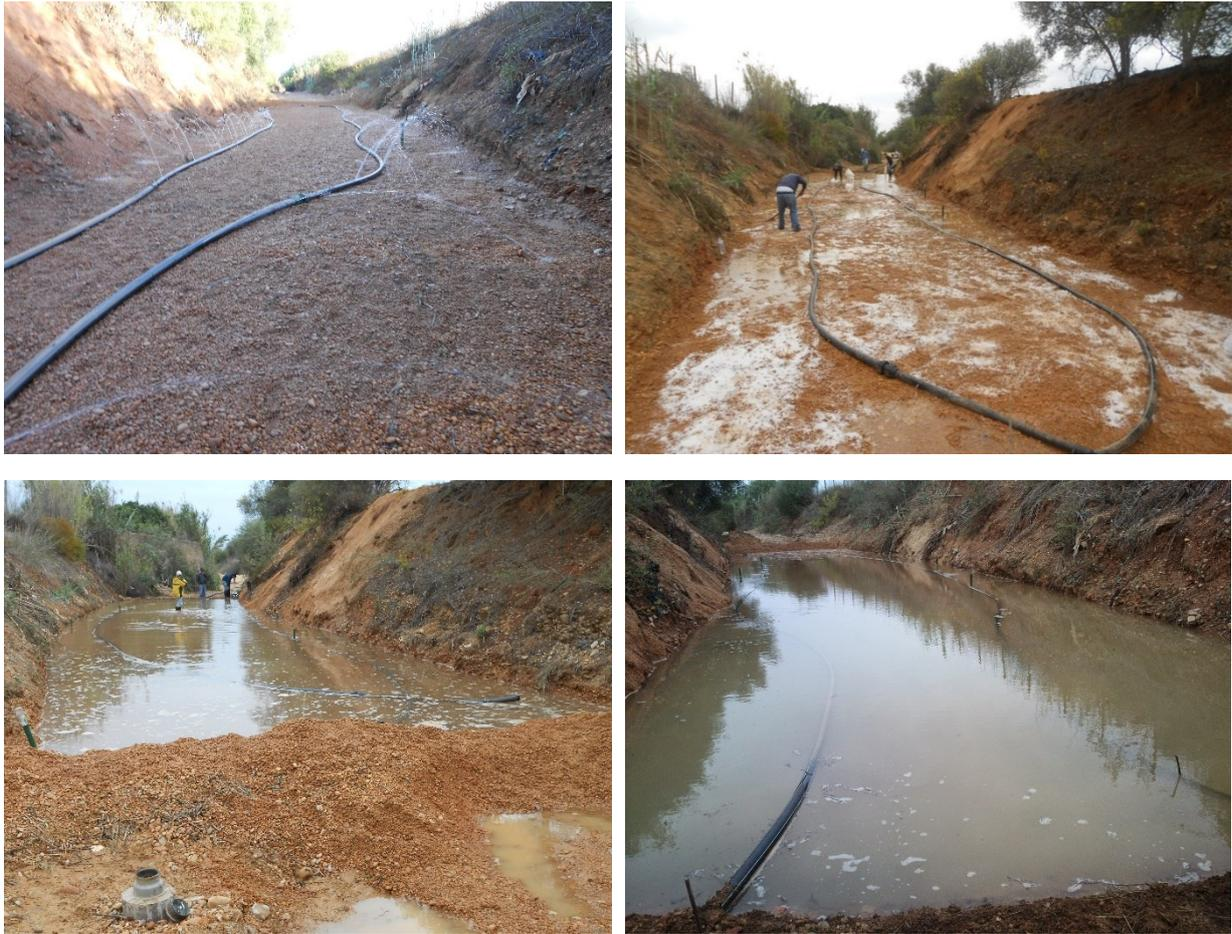
Figure 51 – Tracer test at Rio Seco MARSOL infiltration basin (PT1\_2 Campina de Faro)
