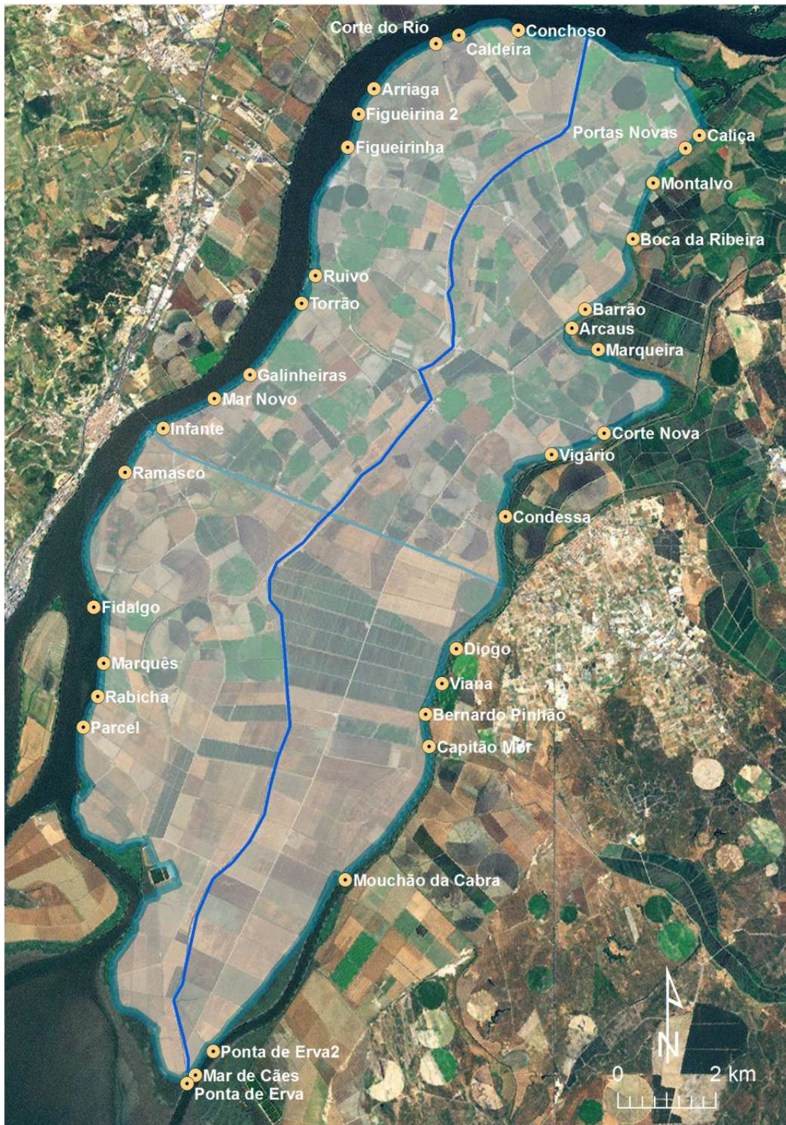
Figure 2.2 – General map of the Aproveitamento Hidroagrícola da Lezíria Grande de Vila Franca de Xira. Main conveyance and drainage channel (blue line) and gates for water intake and drainage – “Portas de Água” (yellow circles). Background image from ESRI basemap. Adapted from ARHT (2009)
