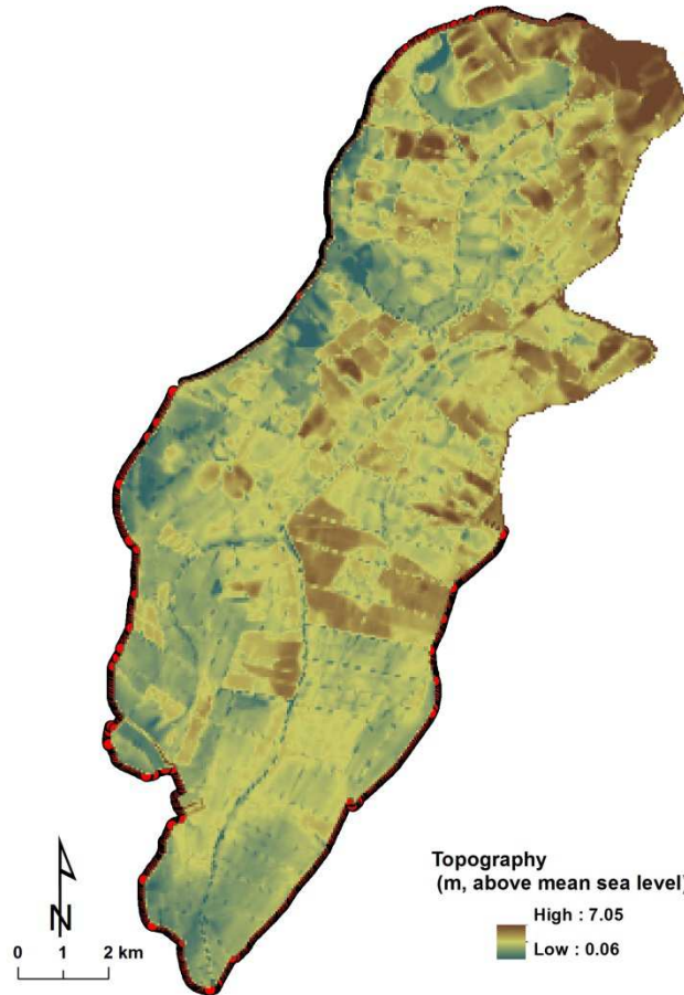
Figure 2.17 –Topography of the Lezíria and dyke crest where the topographic data are available (in red)
