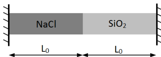
Fig. 4 – Possible geometry of the system considered by Johannessen et al. (1982) to estimate the pressure generated by constrained thermal expansion of adjacent sodium chloride and quartz crystals
