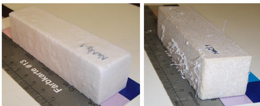
Fig. 7 – Efflorescence of NaNO 3 (left) and NaCl (right) after oven-drying at 105°C
