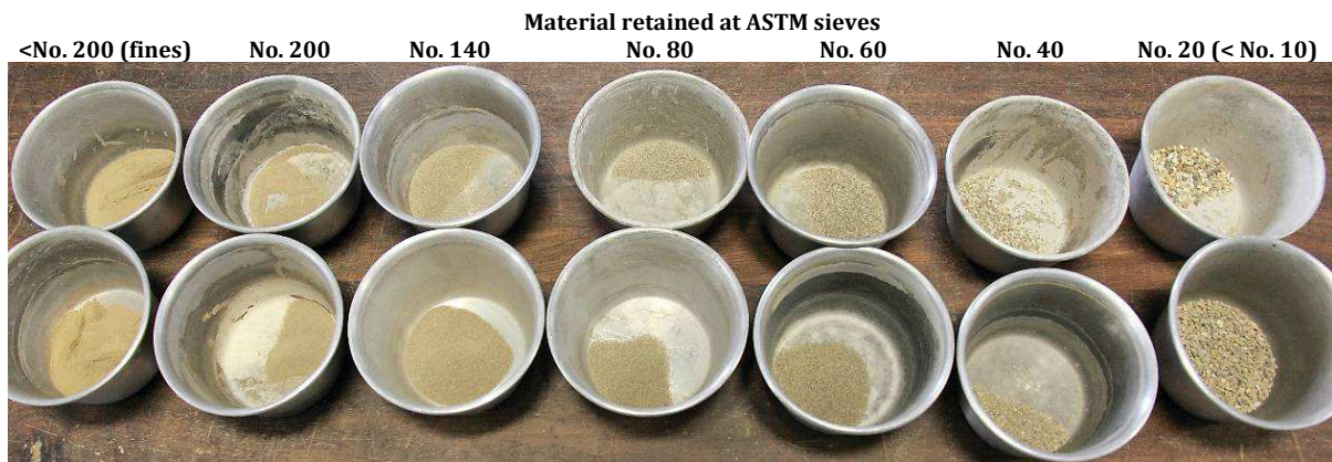
Figure 8.27 – CFETs N1 \cdot G_{wet;D12} (at the top) and N1 \cdot G_{opt;D12} (at the bottom). Total dry material retained at the downstream filter, separated in fractions.
