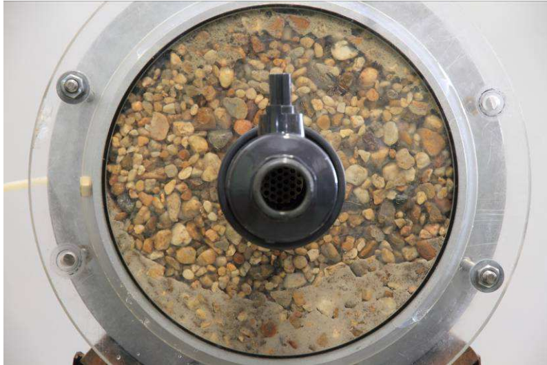
Figure 4.15 – View from the acrylic plate of the downstream filter layer after a CFET. Deposition of soil eroded from the upstream material at the bottom.
