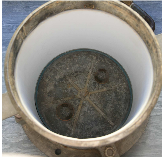
Figure 5.30 – UF test cell used at LNEC, wherein the inner surface of the mould is lined with Teflon® sheet.
