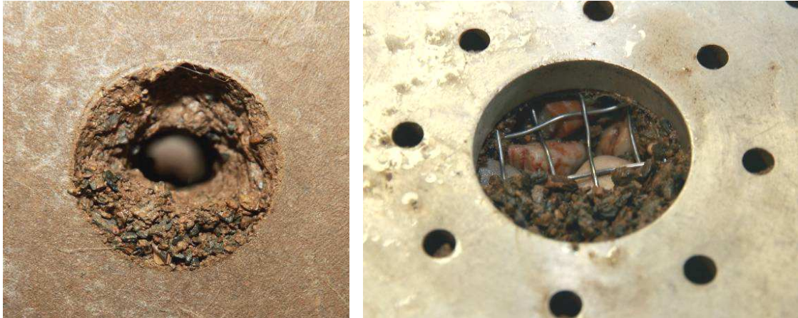
(a) (b) Figure 8.24 – After CFET N1 \cdot G_{opt,D12} : (a) exit of the pipe in the core, and (b) filter face exposed after removal of the core specimen.
