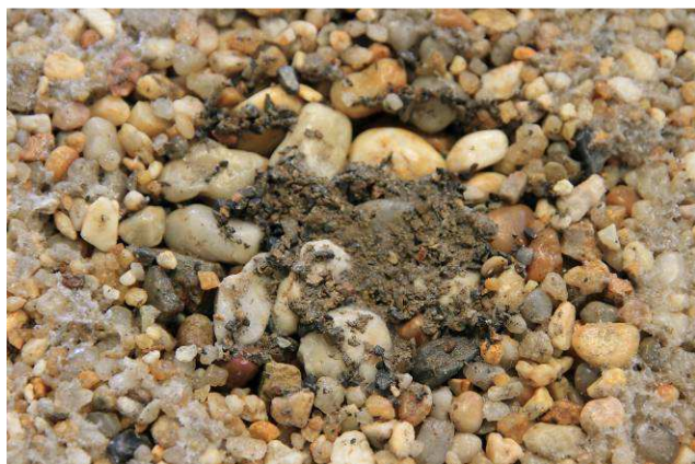
(b) Detail of eroded material accumulated on the filter face at the exit of hole in the core.
