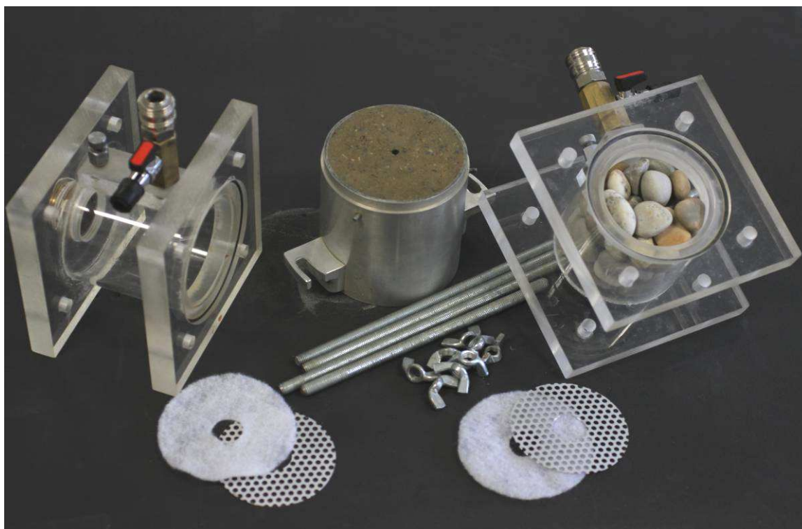
Figure 5.8 – Parts of the test cell of the used HET: specimen of soil compacted inside the mould (at centre), inlet chamber (at right), and outlet chamber (at left).
