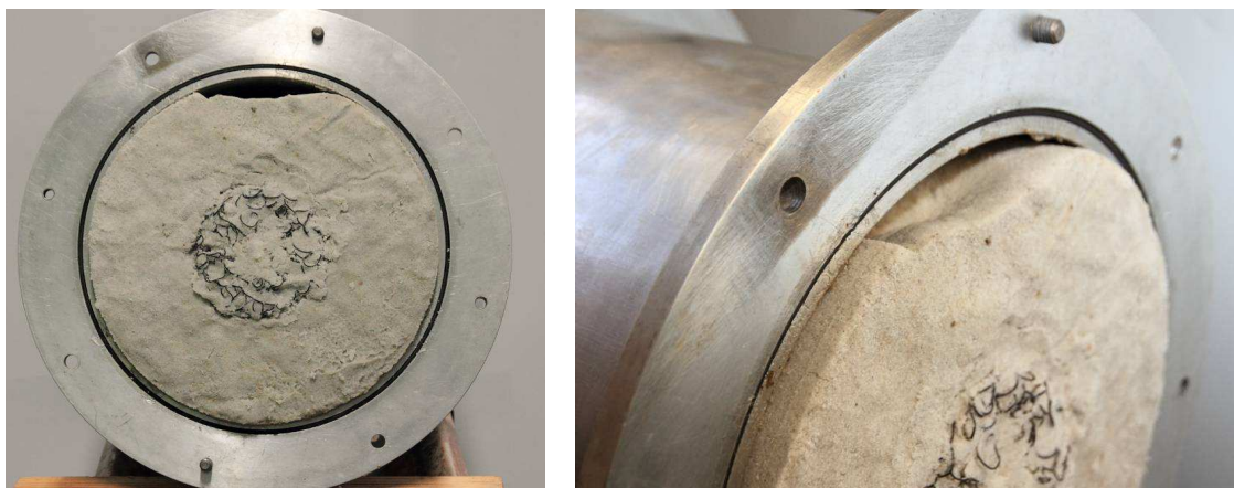
(a) View of the upstream material at the interface with the core.
