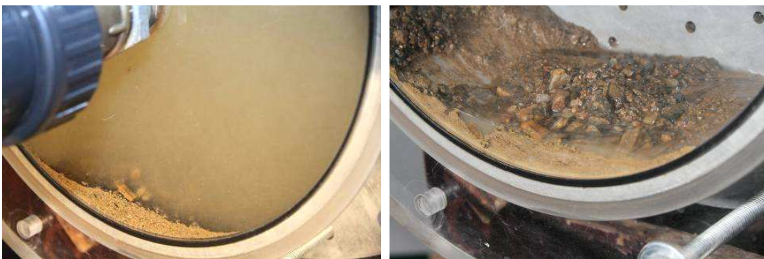
(a) During test, after the blowout of gravel
