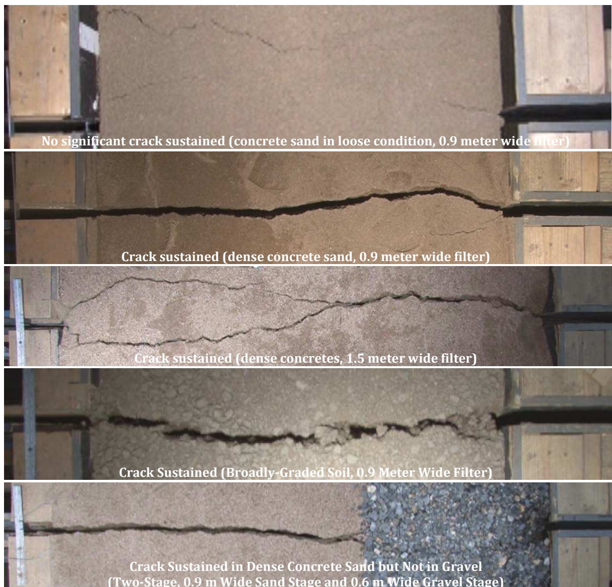
Figure 3.9 - Results of large scale filter testing using 'the crack box' (Redlinger et al. , 2012).
