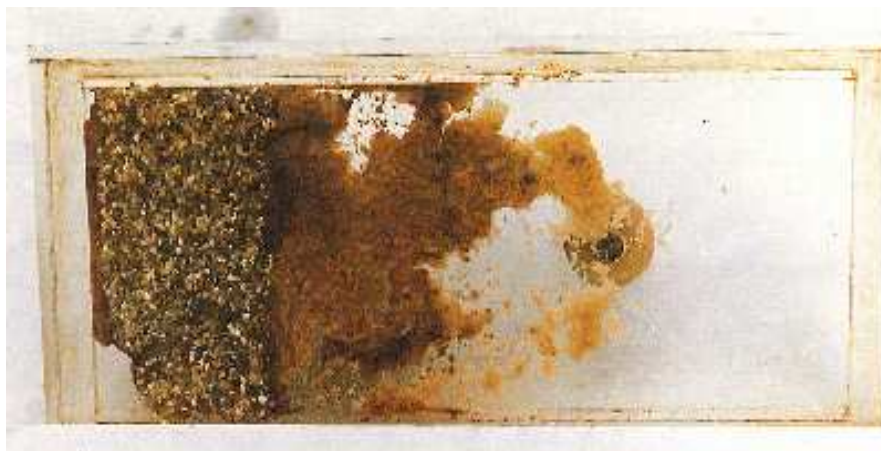
(b) Material adhering to the cover plate when it was removed
