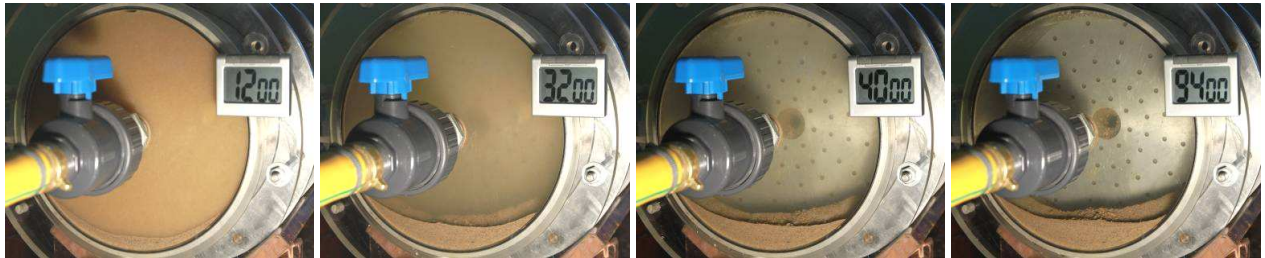
Figure 6.32 – Time lapse (in minutes) of FLET showing behaviour Type 2 (FLET GP_{1w} )
