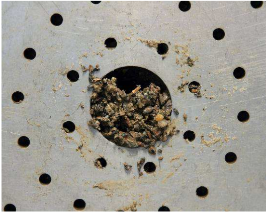
(c) Detail of the material retained at the exit of the hole in the core
