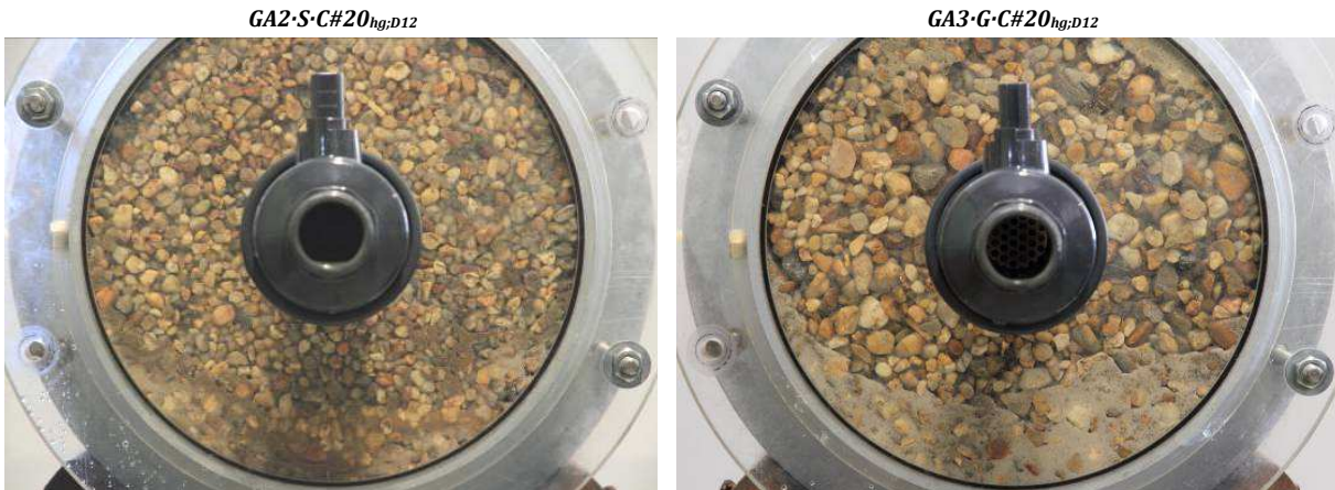
Figure 8.20 - CFETs GA2·S·C#20 hg,D12 (at left) and GA3·G·C#20 hg,D12 (at right). View from the downstream acrylic plate, after emptying the cell.
