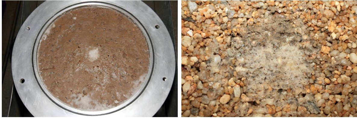
Figure 8.3 - CFET A0\cdot S_{hg;D12} : (at the left) view of the core at the interface with the upstream material (soil A0), (at the right) filter face adjacent to the pipe in the core.
