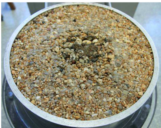
(a) Filter face adjacent to the core
