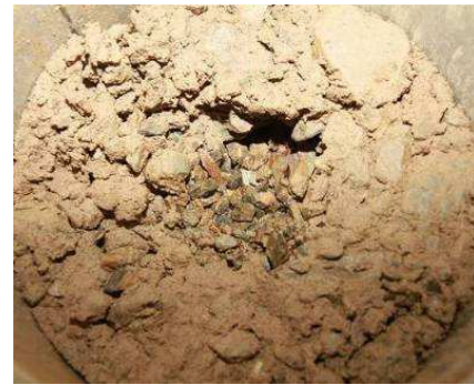
(b) High permeability zone formed in the upstream material, after dismantling of cell
