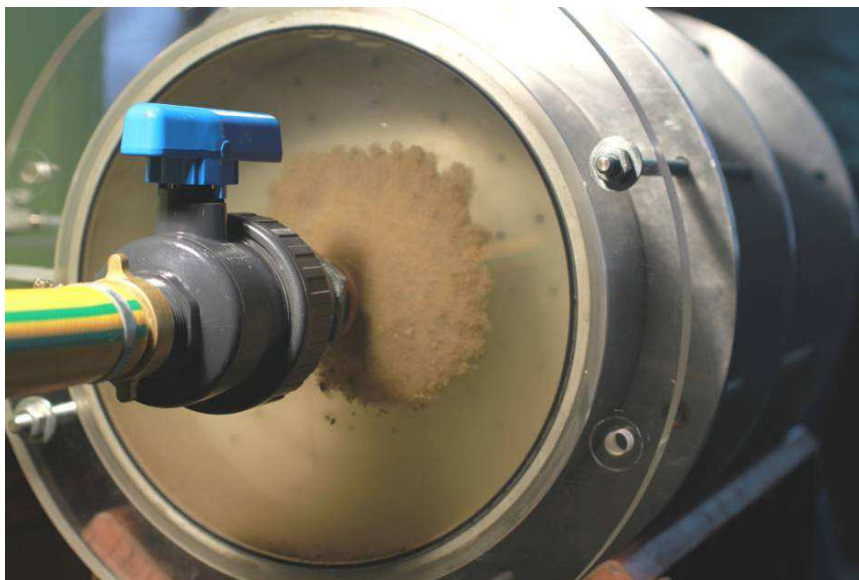
Figure 4.10 – Detail of the test cell from downstream side at the start of a FLET.
