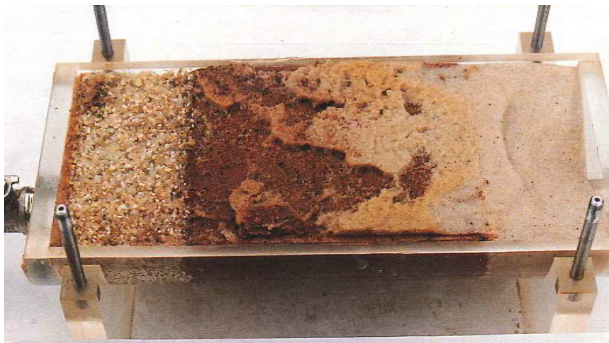
(a) Crack filling with sand (without cover plate)
