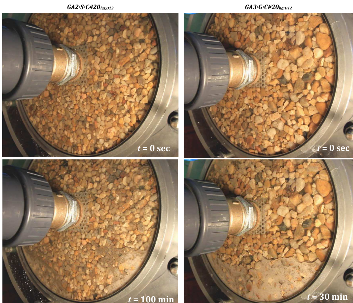
Figure 8.19 – CFETs GA2\cdot S\cdot C\#20_{hg,D12} (at left) and GA3\cdot G\cdot C\#20_{hg,D12} (at right). View from the downstream acrylic plate, at start and towards the end of tests.
