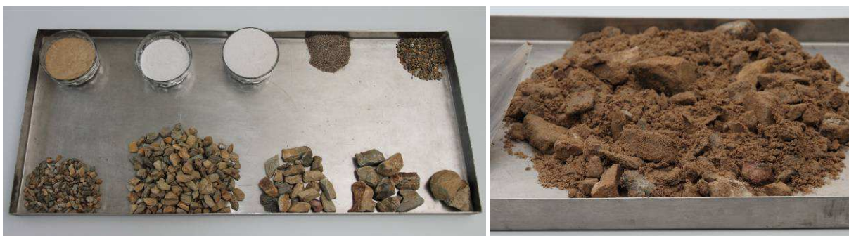
Figure 5.23 – Aspect of soil GN (3 kilograms): soil fractions (at left), and soil mixed with water (at right).
