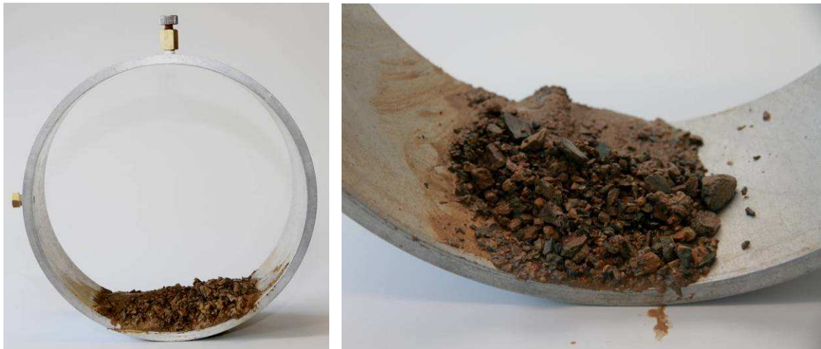
Figure 4.13 - Detail of the eroded material collected in the outlet chamber after a FLET.
