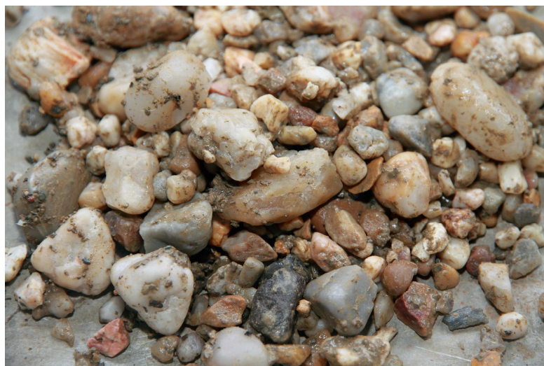
Figure 8.26 – After CFET N1 \cdot G_{wet,D12} : detail of the material collected at the centre of the filter near the pipe exit.
