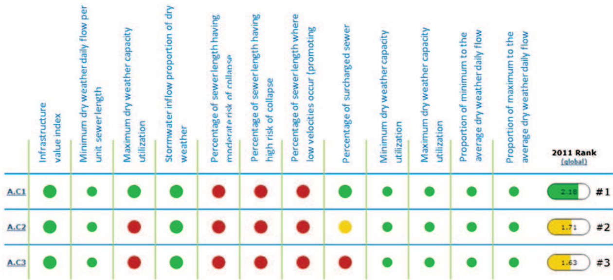
Figure 11. SMAS Oeiras e Amadora scenarios assessment of the current domestic sewer system (Camacho et al., 2012).
