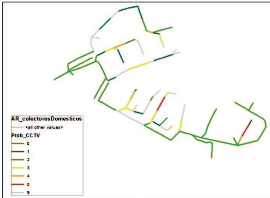
Figure 9. SMAS Oeiras e Amadora structural condition of domestic sewer system (Camacho et al., 2012).
