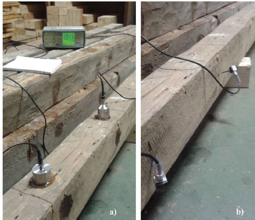
Fig. 2 PUNDITplus (left) and Fakopp (right) transducers applied on the top surface of a timber beam
