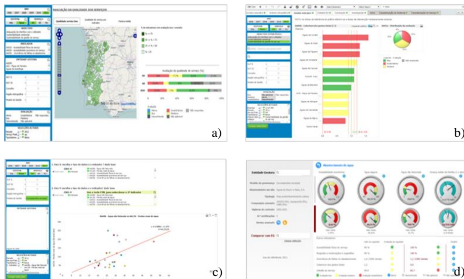
Figure 3. Dashboards of the platform module: (a) Geographical analysis. Quality of service global evaluation. (b) Utilities' ranking and PI assessment. (c) Correlation function. Example: Analysis between non-revenue water and real losses. (d) Reporting's dashboard. Comparison between two water utilities regarding economic accessibility, water quality, non-revenue water and average families' economical accessibility with water service.
