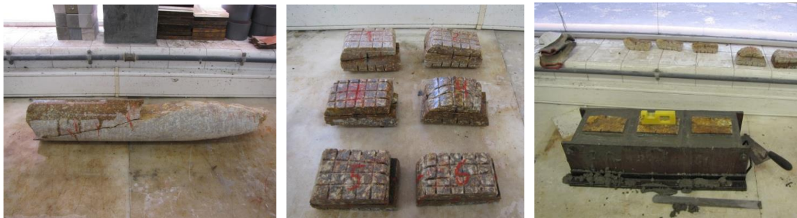
Fig. 2. Specimen preparation: rock core with joint (left); trimmed rock joints (centre); samples being encased in concrete (right).
