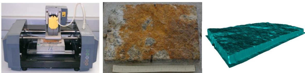
Fig. 1. The scanner with a joint specimen positioned with the Perspex frame, the surface of a rock joint and its corresponding digital image rendered by the scanner control software.
