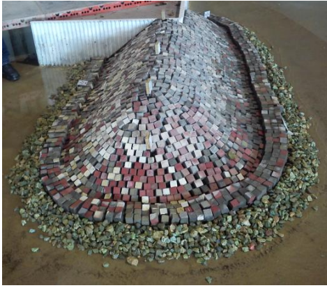
Figure 16 – Model of a breakwater.
