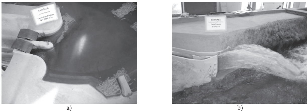
Figure 10. Proposed shapes and design discharge, simultaneous operation ( 3762 \text{ m}^3/\text{s} ): a) control structure, b) ski jump structure.
