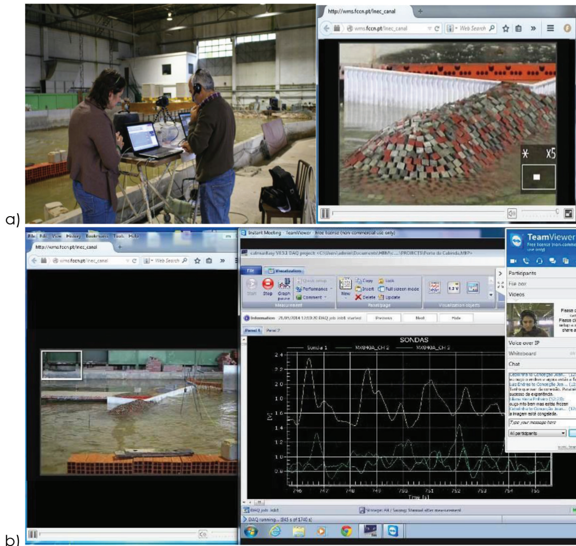
Figure 13: a) Real-time remote visualisation of a model test using image streaming and b) remote access to data acquisition
