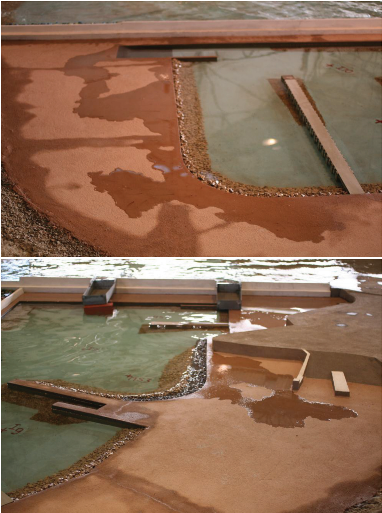
Figure 8: Flooding in some quay areas (Design Solution)
