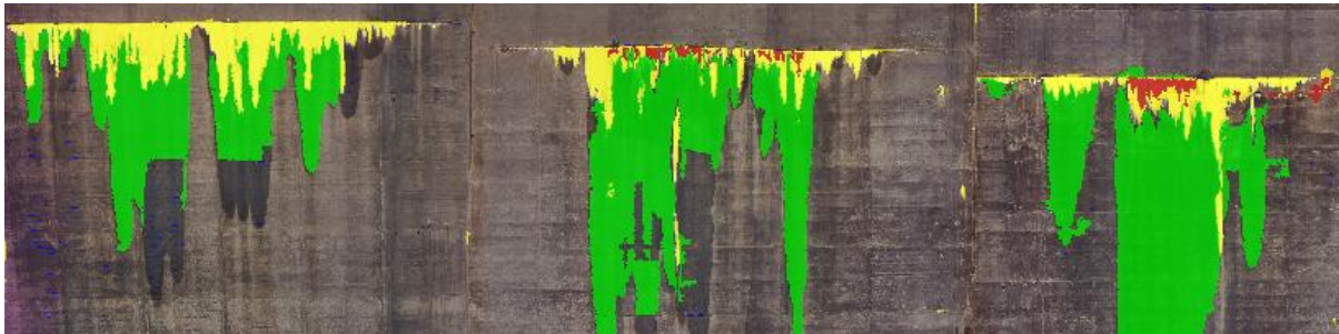
Figure 23: Object-based image classification of the area surrounding the three cracks.
