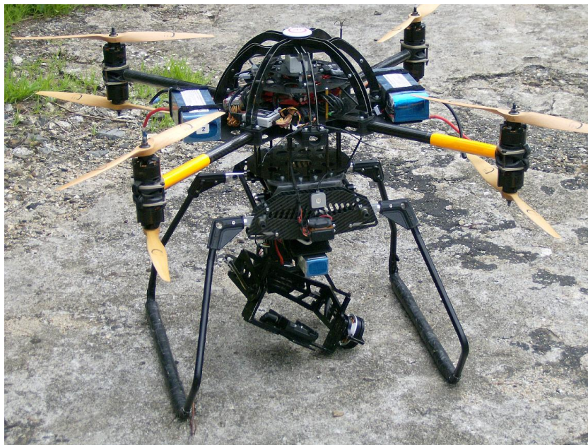
Figure 3: Drone octocopter SKY II. The support of the camera is under the drone, between the landing gears. This photograph was taken before the Sony camera was mounted.
