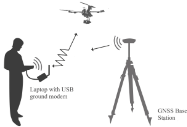
Figure 24: Scheme of communications with a drone with GNSS RTK (adapted from Sensefly).
