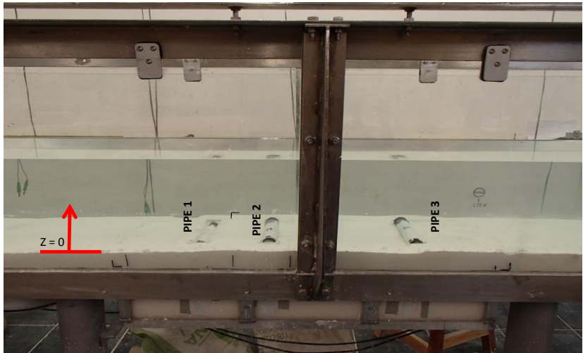
Figure 9. Pipes in the flume at the beginning of the tests.
