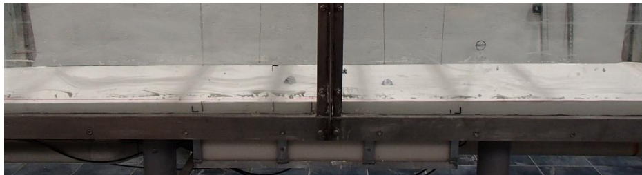
Figure 8. Flume during the preliminary tests (top) and with the soil tray enlarged and with the three structures semi-fixed to reduce the horizontal movements of the pipes (bottom).
