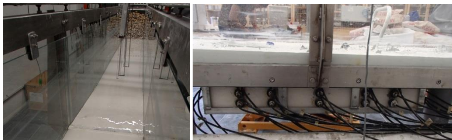
Figure 3. Aspects of the flume with the equipment used in the tests: wave gauges and pressure sensors.
