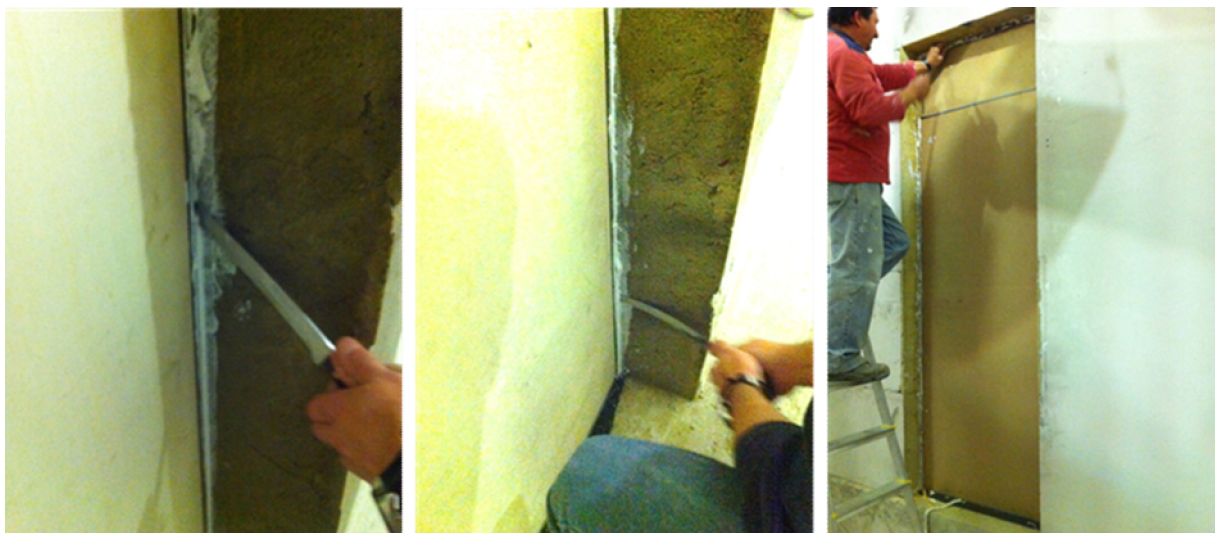
Figure 4 – Cutting of silicone in order to remove the sample from the opening.
