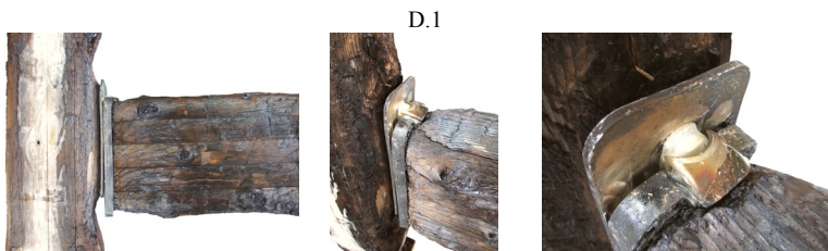
Figure 12. Connection D.1 after the fire test.
