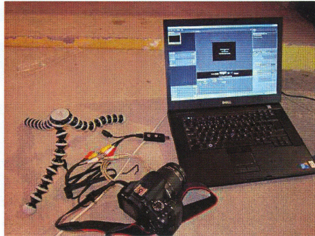
Figure 2. Equipment used during the remote access experiment. Laptop computer, A/D Converter DAQ board, cables with USB-composite video adapter, a Canon camera and a flexible tripod.
