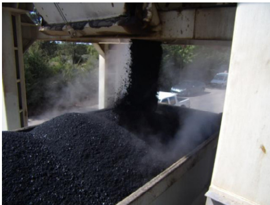
Fig. 3. Exit of the WMRA to the trucks
