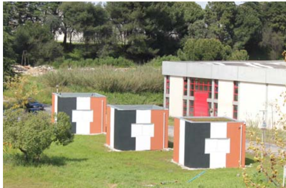
Figure 1: Full-scale test cells painted with three different reflective paints
