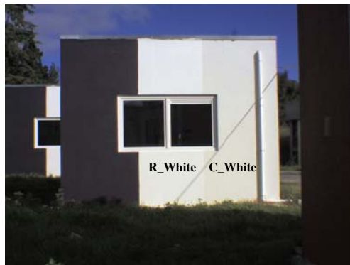
Figure 3: Test cell with Conventional White (C_White) and Reflective White (R_White) paints
