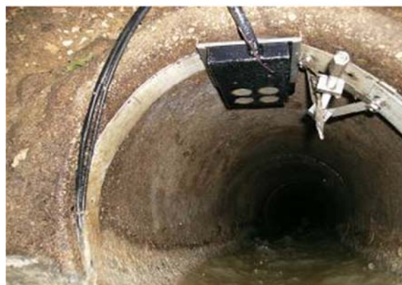
Figure 5.3: Flow measurement device: detail of ultrasound device (four pairs) for flow depth measurement
