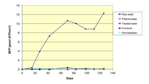
Figure 6-1 Biofilm formation in water after various treatments at the Oset plant
