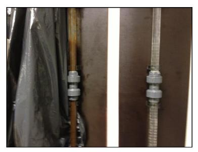
*Figure 6-2 The effect of NOM removal on the biofilm formation: biofilm grown in raw water (left) and in filtered water (right)*
