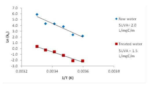
*Figure 7-1 Arrhenius plot showing the influence of temperature on chlorine bulk decay coefficients*
