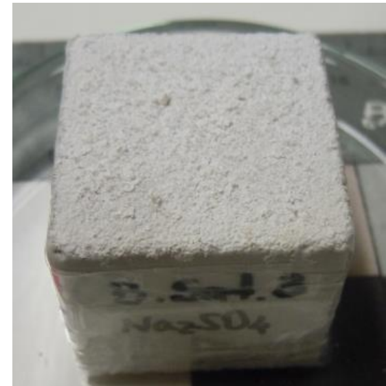
Surface alteration: efflorescence
