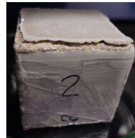
Grey limestone uni-layer delamination
