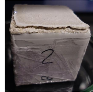
Grey limestone uni-layer delamination
