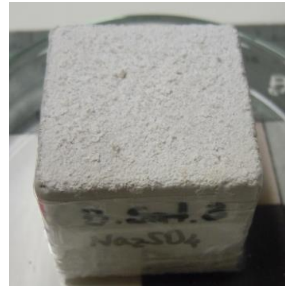
Surface alteration: efflorescence
