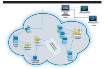
Figure 1. Physical architecture of the RDFS. Adapted from Jesus *et al.*, 2012.
