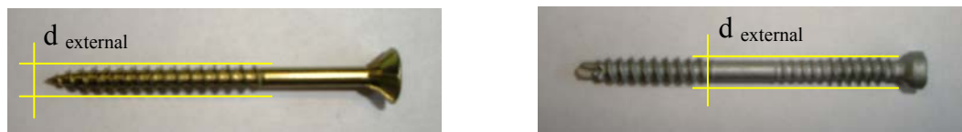
Figure 1: a) Common screw 5.0x60 ( d_{ext}=5.0 mm; d_{int}=3.1 mm), b) SFSintec WT-T4,5 ( d_{ext}=4.5 mm; d_{int}=3.3 mm)
