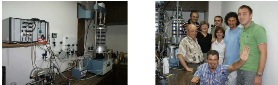
Figure 4. Installed tri-axial system and training of the laboratory staff
