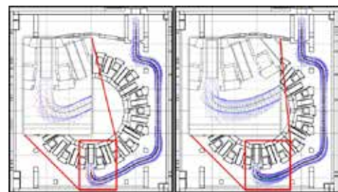
Figure 9: Comparison of non feasible trajectory using line guidance (left image) and the a feasible trajectory using free roaming (right image) to port 14 in level B1 of TB.
