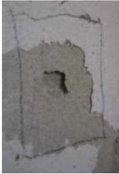
Fig. 19 –HMC at 95% of different layers of the render (left) and picture of one of the sampled areas showing the different layers (right)
