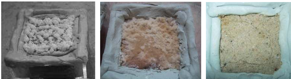
Fig. 5.9 - Preliminary crystallization tests by continuous immersion on lime-plaster/brick specimens. Abundant efflorescence occurred under all environmental conditions both for the 1.9 molal sodium chloride (on the left) and the 0.39 molal sodium sulfate (on the centre) solutions. Its removal systematically revealed wet undamaged plaster surfaces. The only exception were the tests with high temperature periods (constant or cycles) on sodium sulfate, where cracking of the specimens was observed (on the right).
