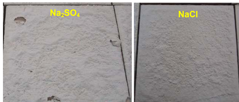
Fig. 5.36 - Damage on the acrylic paint at the end of the first crystallization experiment
