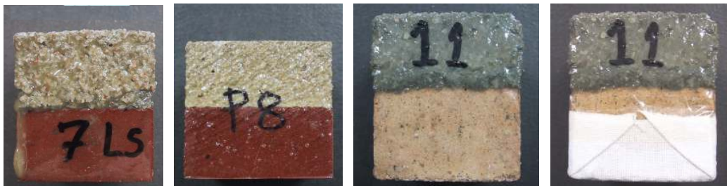
Fig. 5.10 - Specimens (side view) used in set 1 tests: LNEC on brick (specimen 7LS), Parlumière on brick (specimen P8) and LNEC on lime mortar (specimen 11) without or with protective tissue
