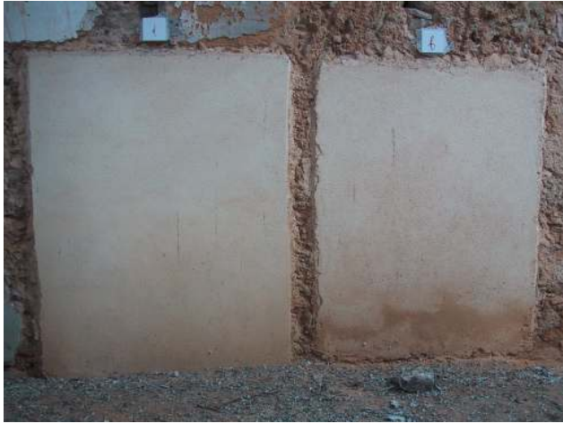
Fig. 5.2 – Test panels on the interior of S. Sebastião church, Almada, one year after their application. Each panel is made of two similar plaster coats composed by a mortar with volumetric composition of 1:1.5:1.5 (dry-hydrated lime: sand from Tagus river : yellow pit sand from Corroios). In the panel on the right a commercial air-lime with hydrophobic properties was used. In contrast to the panel on the left, where ordinary air-lime was used, more severe dampness and sanding of the mortar at the base of the panel were observed here.
