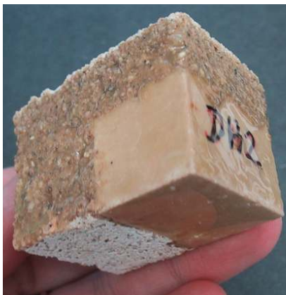
Fig. I.7 – Test-specimen made of plaster on mortar/stone substrate
