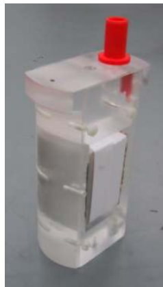
Fig. I.8 - Sample-holder with specimen inside
