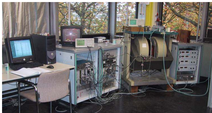
Fig. I.6 – NMR set-up for 2D measurements at TUE composed by, from left to right: computer; data acquisition and RF transmitter; RF receiver; electro magnet; power supplies.
