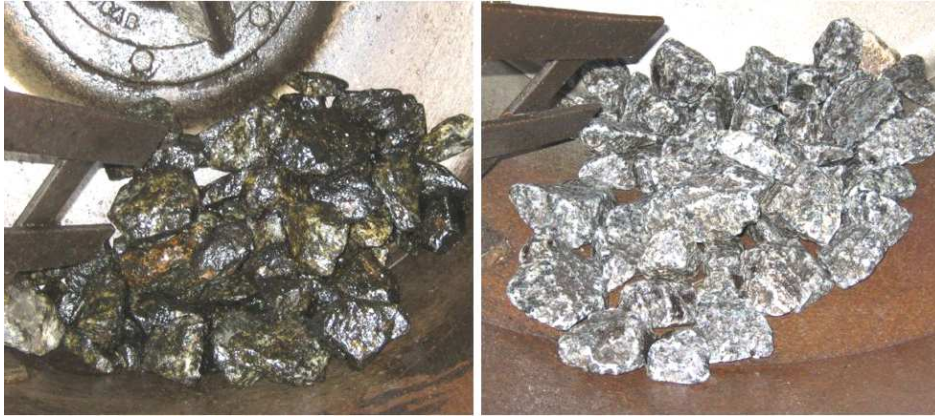
Figure 1 – Comparison Between Ballast Before and After the Procedure Wash with SOLV-LAT 10%.
