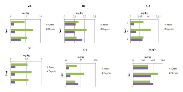
Figure 6 – Results on soil samples leachates, collected before and after nZVI injection at zone III.
