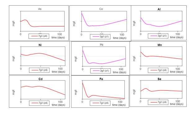
Figure 5 – Summary results on water samples, collected before and after nZVI injection in zone I, II and IV.
