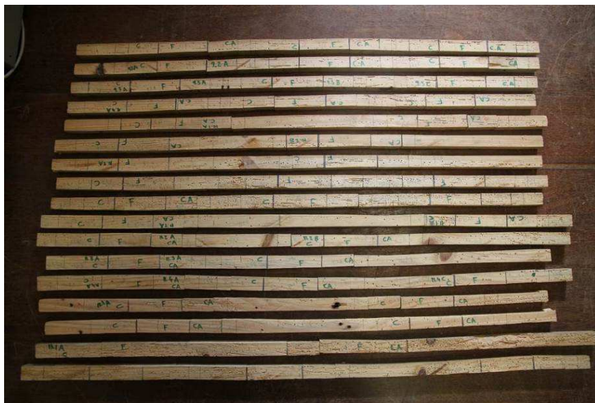
Figure 2. Some of the fascia used for bending and compression tests
