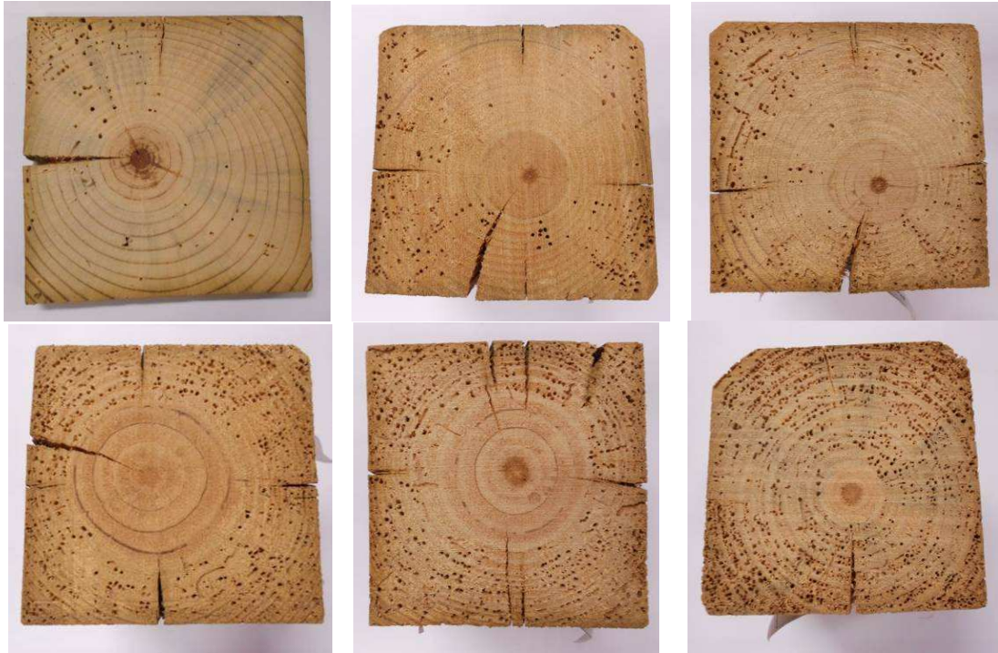
Figure 1. Diffuse beetles attack (cross sections of 12cm x 12cm approximately)
