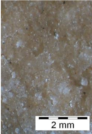
Fig. 15 Thick, compact and vitreous NaCl crust of irregular texture with isolated salt crystals: 30x magnification of B.20.2 specimen
