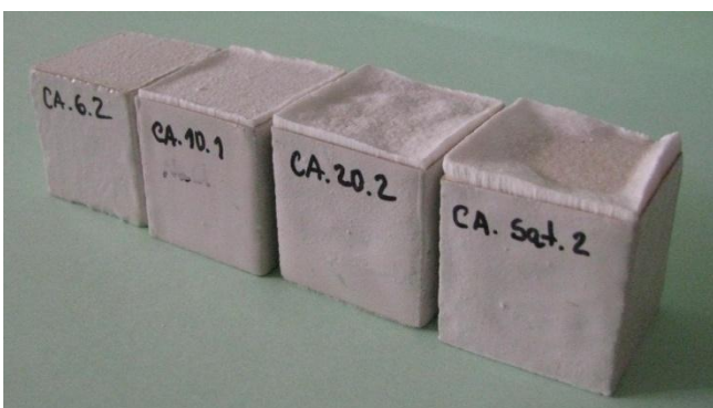
Fig. 8 The thickness of the \text{NaCl} crust on Ançã limestone increases with the concentration of the salt solution (from left to right) and shows a preferential deposition at the edges of the specimens
